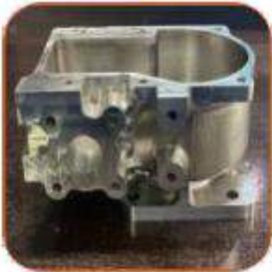
Actuator Body (Copper Nickel Alloy)
