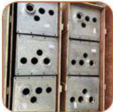
Aluminum Castings LM 10 Kavach MOD -II assembly part
